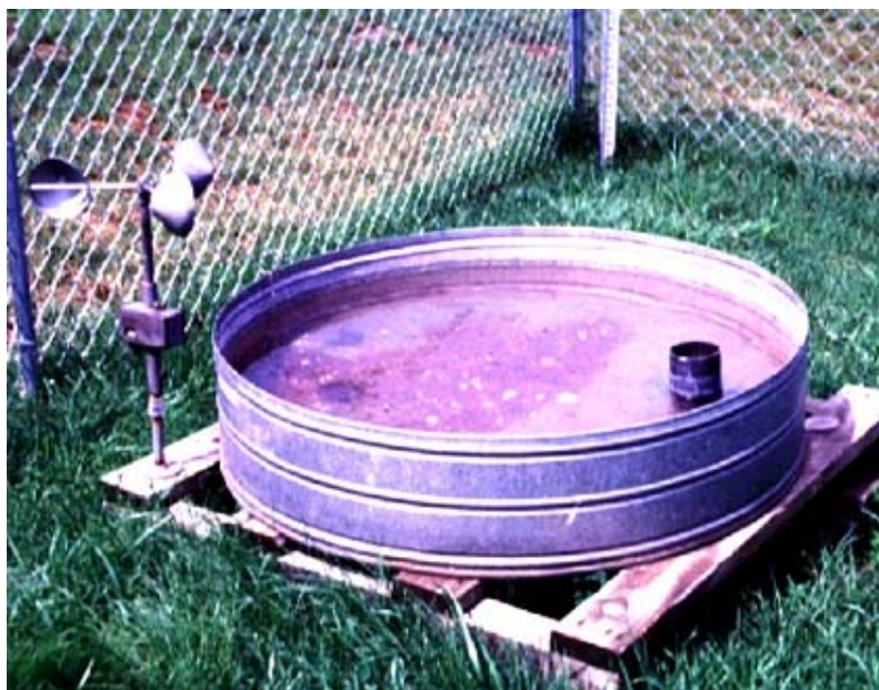
In the picture: USWB Class a Pan Evaporimeter for Estimating ET_o
