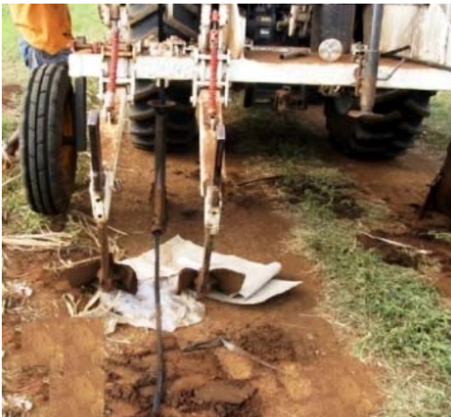
In the picture: Subsurface dripline laying machine
